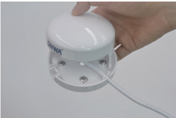
4. Run the cable through the hole on the base.
