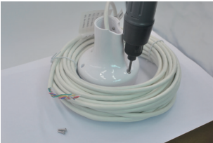
3. Use screws to tighten the mounting base to ensure a secure installation.
