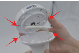
1. When installing, align the two clips with the corresponding slots.
