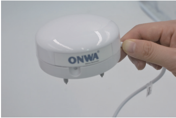
5. After placing the GNSS Antenna on the base, rotate the knob to the right to tighten it.
