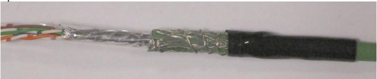
*Picture showing how to make the cable on board if shortened*
